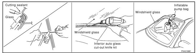
7. Remove the windshield glass, using suction.
