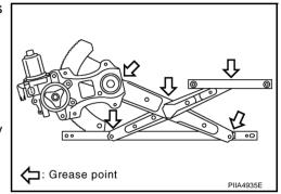
Disassembly and assembly REGULATOR ASSEMBLY
