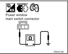
4. Check continuity between front power window switch (passenger side) connector D36 terminal 11 and ground.
